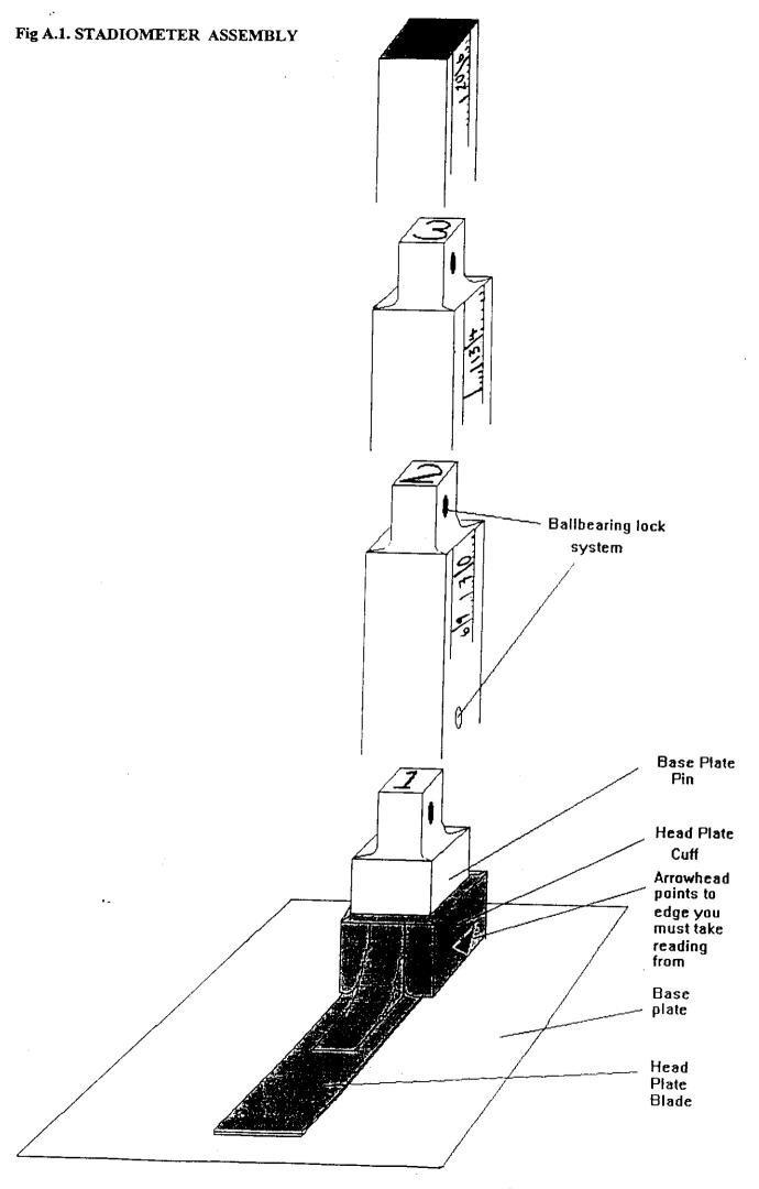
pressure. Grasp the head plate by the cuff whenever you are moving the headplate up or down the rods, this will prevent any unnecessary pressure being applied to the blade which may cause it to break.
