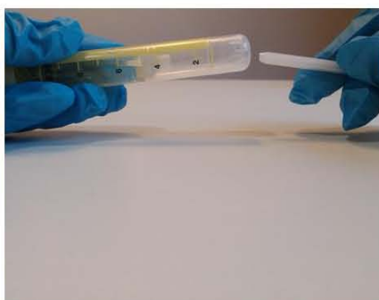
6. Break off the stalk of the plunger
