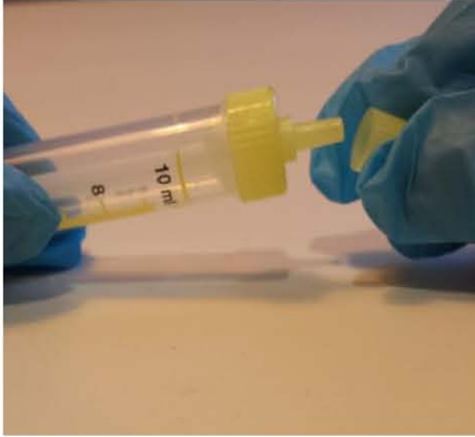
1. Remove the small push cap.
