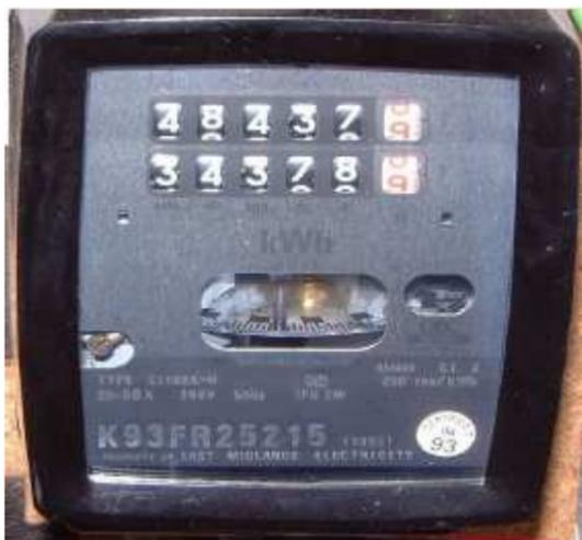
If the meter has two rows of numbers marked Low (Rate 1) and Normal (Rate 2) write them in the *Low (Rate 1)* and *Normal (Rate 2)* sections in CAPI.
