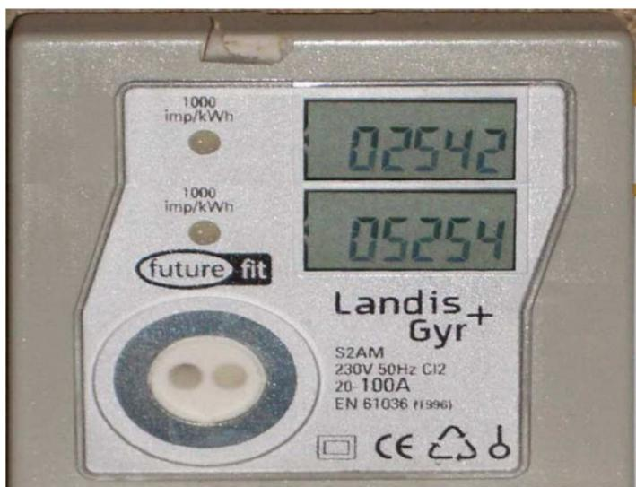
If the meter has two LCD screens marked *Low (Rate 1)* and *Normal (Rate 2)*, write down the lower number where prompted and the higher number where prompted in CAPI.
